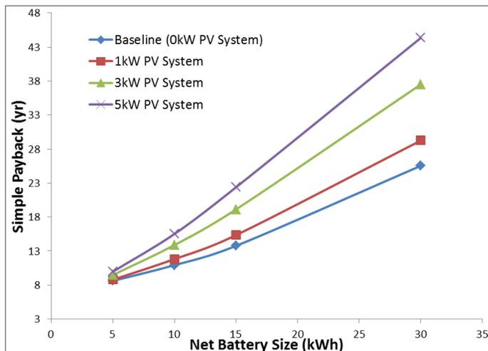
Figure 11: Simple Payback of Battery Sizing with PV system (Scaled Case)
