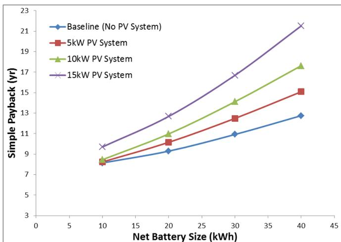
Figure 10: Simple Payback of Battery Sizing with PV system (Base Case)
