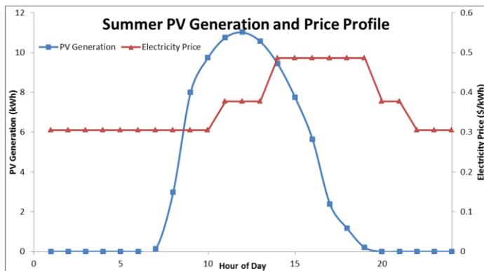
Figure 2: Correlation of TOU rate structure with solar PV production during summer months
