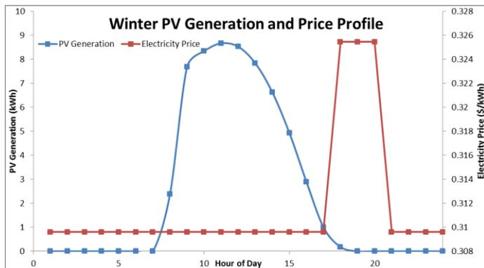
Figure 3: Correlation of TOU rate structure with solar PV production during winter months
