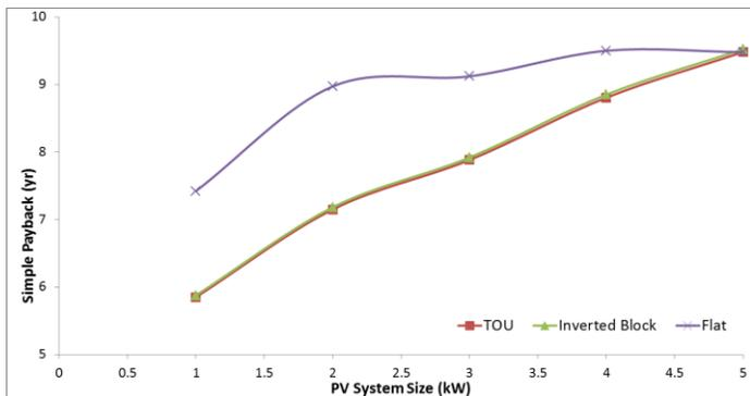
Figure 8: Simple Payback of PV systems for Common Rate Structures (Scaled Case)
