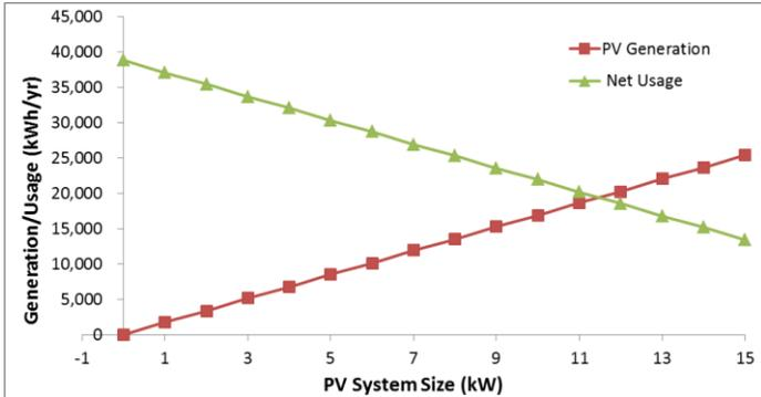
Figure 4: Solar PV Generation and Net Consumption (Base Case)
