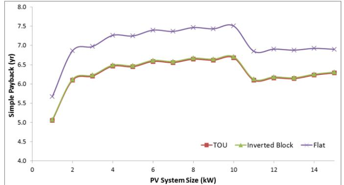
Figure 6: Simple Payback of PV systems for Common Rate Structures (Base Case)
