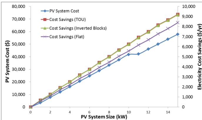
Figure 5: Annual Costs and Savings of Solar PV Installation for Common Rate Structures (Base Case)
