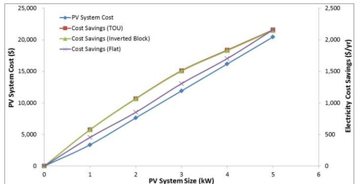
Figure 7: Annual Costs and Savings of Solar PV Installation for Common Rate Structures (Typically-sized Case)
