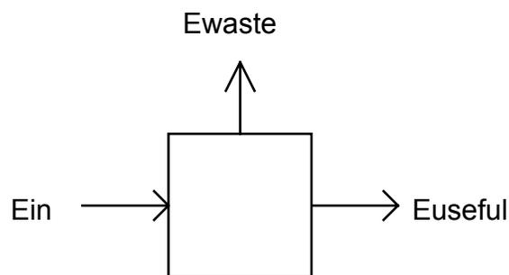
Figure 2. Energy flows entering and exiting a typical energy conversion device such as a furnace, boiler, motor or engine. *Journal of Strategic Planning for Energy and Environment*, Association of Energy Engineers, Vol. 21, No. 1. 2001. 2
