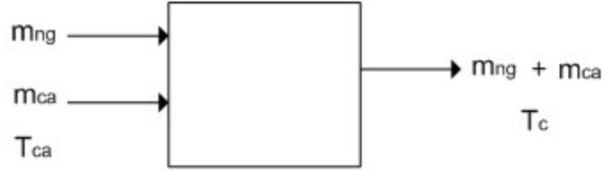
Figure 2. Mass balance on combustion chamber
