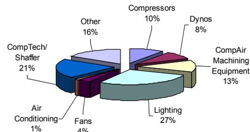
Figure 7. Example of electricity use breakdown by equipment.
